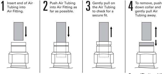
**Removal Tip:** Use a 1/4", 5/16", or 6mm open-ended wrench to push the collar down.
