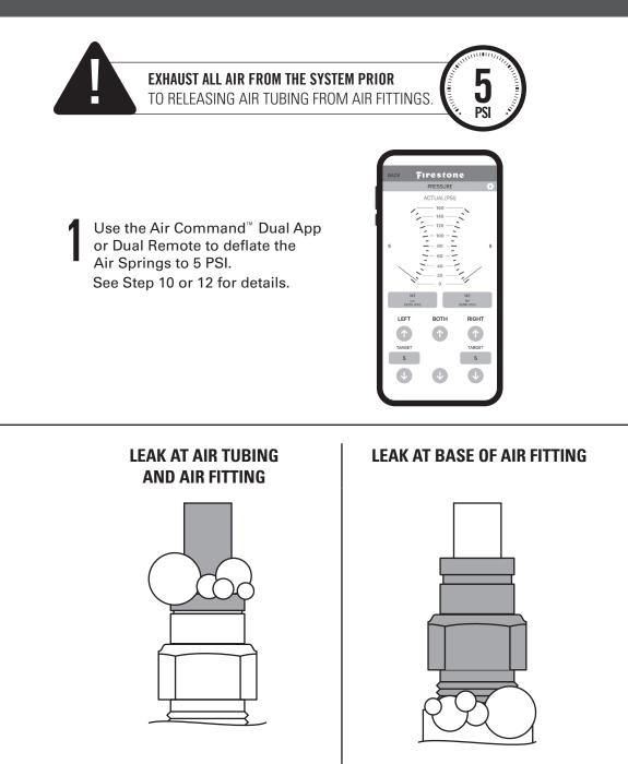
Release AirTubing (see page 4). Review proper cuts and procedures in Step 5. Repeat Step 5. Tighten Air Fitting one turn or until leak stops.
