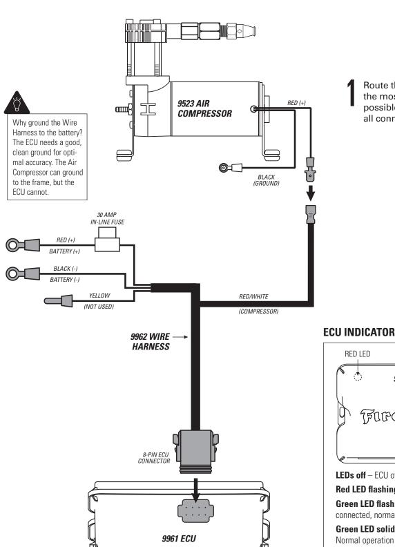
Route the Wire Harness in the most protected manner possible, and securely make all connections as shown.
