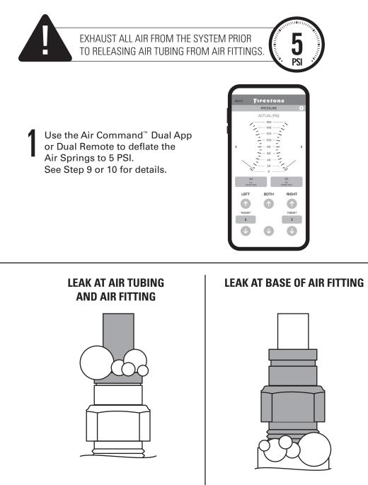
Release AirTubing (see page 4). Review proper cuts and procedures in Step 5. Repeat Step 5. Tighten Air Fitting one turn or until leak stops.
