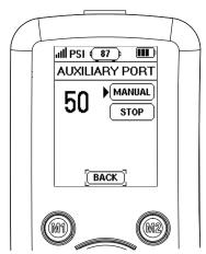
Manual Mode, when selected, will run the compressor until the user presses the stop button. Measured pressure is shown on the left.
