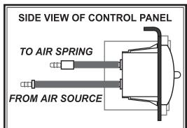
To inflate the air springs, simply push the paddle up until the desired air pressure is reached.
