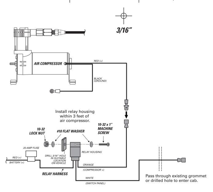
Connect wires, install ring terminals and wire connectors as shown below.
