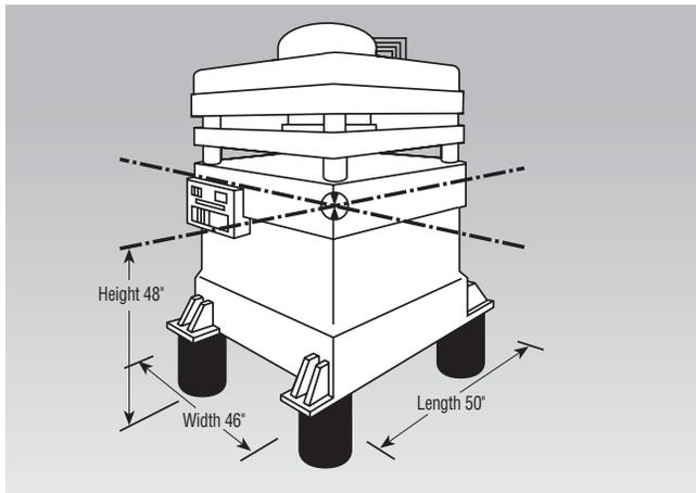
In the above example, the most narrow distance between two Marsh Mellow springs is 46 inches (117 cm). The height to the CG is 48 inches (122 cm); therefore, this system does not meet our guideline. Two possible solutions would be:
